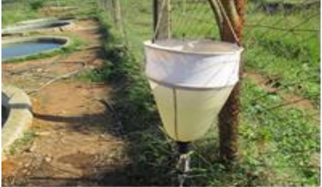
Figure 3.2 Concentrating the water sample using plankton net
