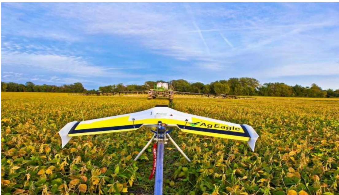
Figure 3. Agrobotix drone: a low-cost crop data tool for farmers, over time, or in real-time, equipped with infrared sensors
