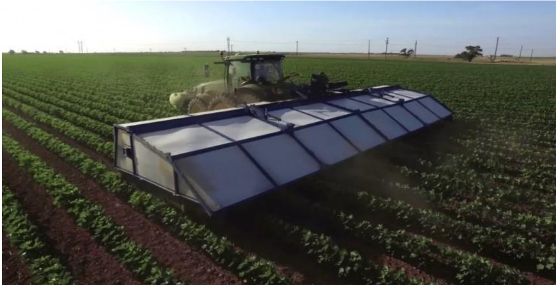
Figure 2. Robot attached to a tractor to thin out lettuce fields and prevent herbicide resistant weeds
