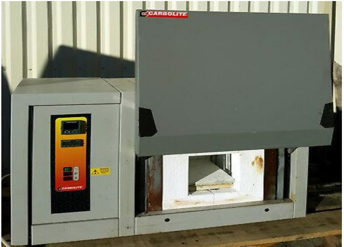
Plate 3.1 Carbolite HT F17/5 High-Temperature Laboratory Chamber Furnace (5 litres 1700°C)
