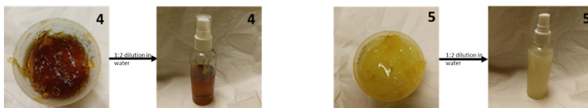
Figure 2: Liquid soaps produced from 7:2:1 ratio of C. megalobotrys , R. cummunis and Coconut seed oils (4) and 10:1 ratio Sunflower and Coconut seed oils (5 (control)).
