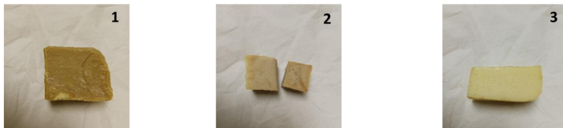
Figure 1: Solid bar soaps produced from 10:1 ratio of C. megalobotrys and Coconut seed oils (1), 7:2:1 ratio of C. megalobotrys , R. cummunis and Coconut seed oils (2) and 10:1 ratio Sunflower and Coconut seed oils (3 (control)).
